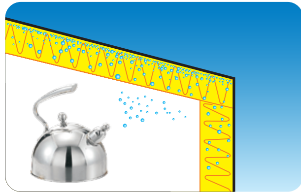
Poor Quality Insulation Facing
